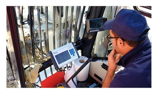
**CFA VISION** measurement system is a logger device for the drilling and grouting parameters applied to the technology of continuos flight auger (CFA) device based on Windows CE unit with a 7" color display.
