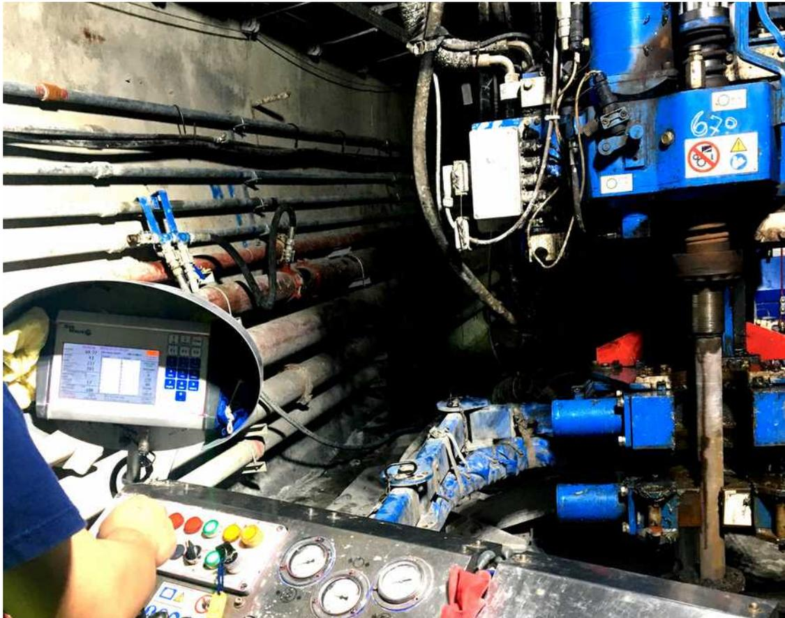
**FORA-VISION** measurement system is a read-out and sensor device for the drilling parameters used in **perforation technology (DAC test)**.
